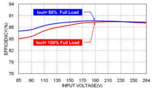
43MAD30US24B Efficiency vs. Input Voltage
